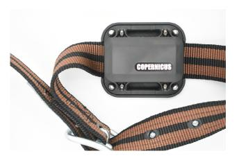
The LoRaWAN GPS tracking collar 'Bull' allows tracking of animals over a prolonged period. Due to the light weight of the device, various adult species can be monitored with an appropriately sized collar. Thanks to the devices' internal data storage capability, migrating individuals can be tracked all year around without data loss.
