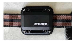
The LoRaWAN GPS tracking collar 'Bull' allows tracking of animals over a prolonged period. Due to the light weight of the device, various adult species can be monitored with an appropriately sized collar. Thanks to the devices' internal data storage capability, migrating individuals can be tracked all year around without data loss.
